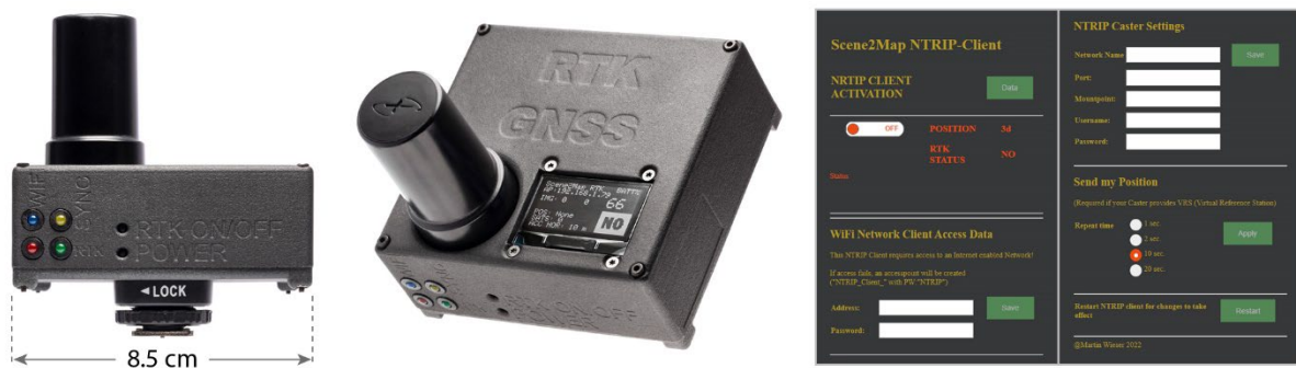
Figure 8 – The new RTK-enabled GNSS-IMU logging device (left and middle) with the interface controlling its settings (right).
