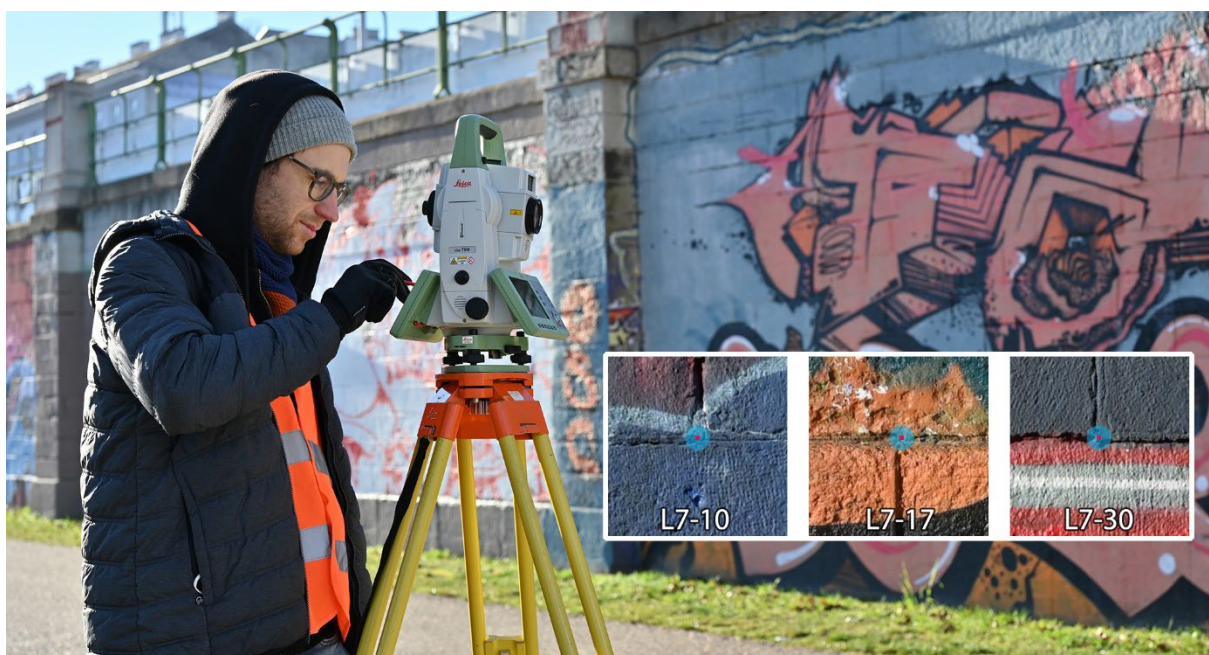
Figure 10 – Benjamin Wild operating the Leica Viva TS16 total station. The inset on the lower right displays three typical GPs.
