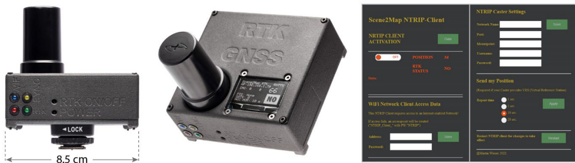
Figure 14 – The new RTK-enabled GNSS-IMU logging device (left and middle) with the interface controlling its settings (right).
