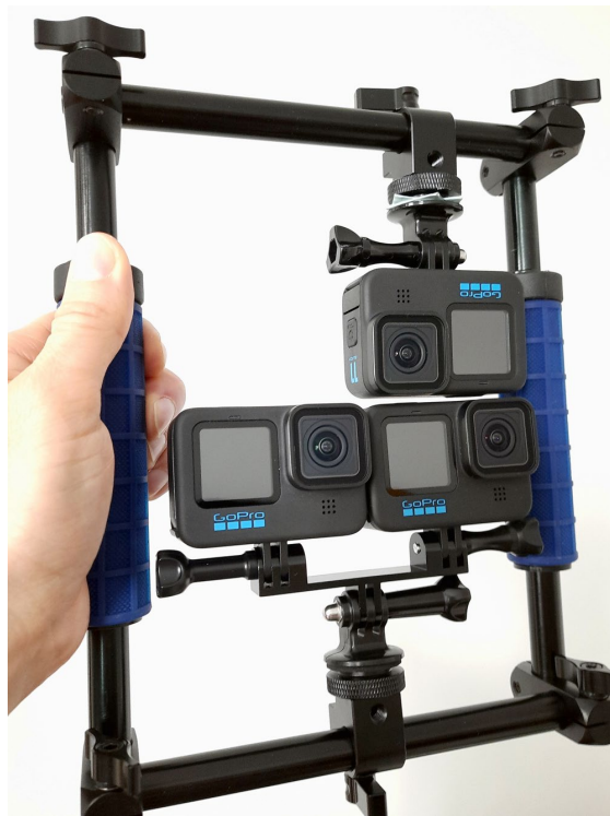
Figure 23 – Three GoPro cameras mounted inside a frame composed of standard camera rig components.
