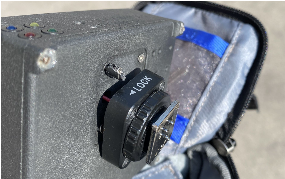
Figure 15 – RTK GNSS device B with the broken connection part (photo by Stefan Wogrin).
