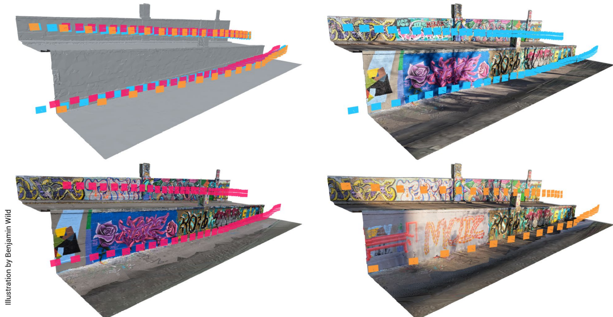
Figure 24 – The upper left image shows the position of INDIGO's GoPro HERO11 black photos acquired on three days. The same 3D meshed surface model of the test zone can be textured with these photographs to yield epoch-specific textures. Illustration by Benjamin Wild.
